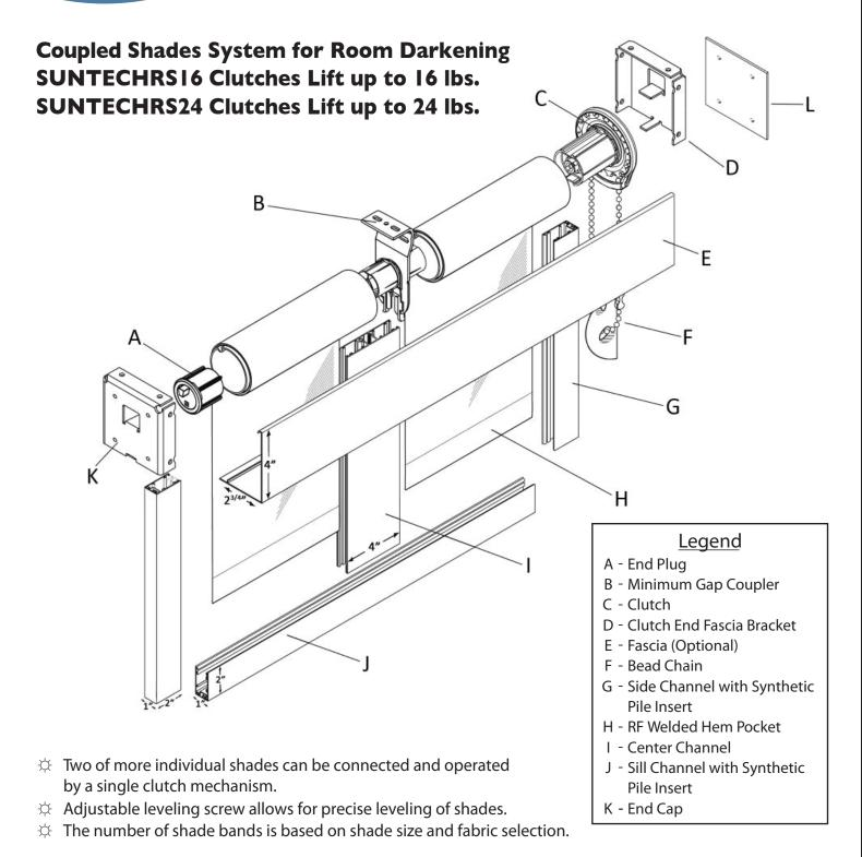
Side and sill channels and center channel are extruded aluminum with synthetic pile inserts to eliminate light leakeage.
